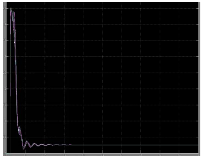
Fig. 5: Active power without filter
